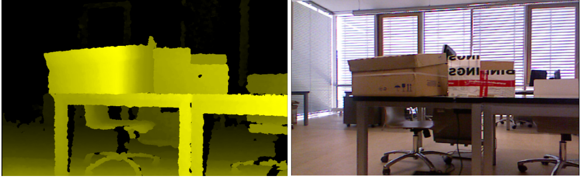
Figure 1: Left image represents the Kinect depth image, the black pixels have unknown depth value, mostly because of occlusion or reflective surface material. Right image is captured by Kinect RGB camera.
